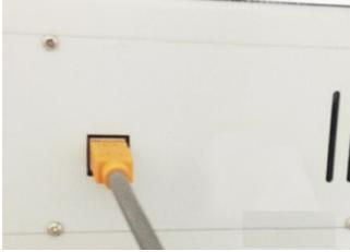
As shown on the left, connect one end of the video cable to the device and the other end to the USB port. Then on the basis of 5.2, to install the video driver.
