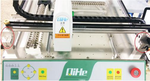
Place the machine as the position of left picture, check whether the gap in two circle rings are unanimous with your picture in the disk. If not unanimous then means happen tooth jump appearance.◦
