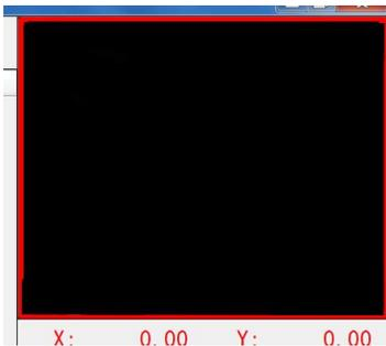
Shown as right picture, the video window are dark, no circle ring and cross, this means video wire not connected well, or drive isn't installed well.
