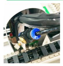
Shown as left picture, 22 is the air blow adjust valve, it locate at back of mounted head. The air blow adjust valve formed with adjust button, lock nuts and cave body. When adjusting, first loosen the lock nut then twist the adjust knob, clockwise rotating is reduce the air blow volume, anticlockwise rotating change to increase air blow volume, the users adjust the air blow volume according to actual situation.
